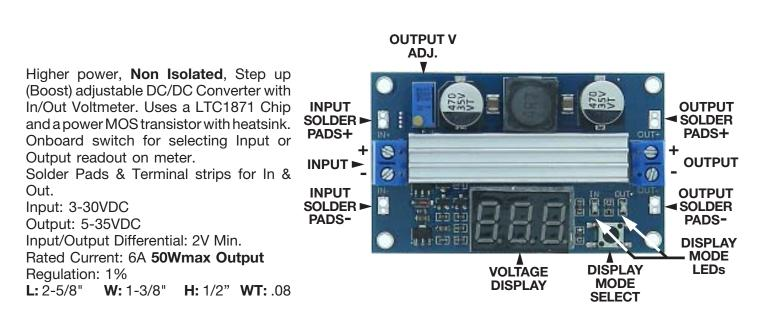
**NOTE:** INPUT & OUTPUT - (Minus) are common (Connected together) Respective Input Solder Pads & Terminal Strip Connections are the Same Respective Output Solder Pads & Terminal Strip Connections are the Same
