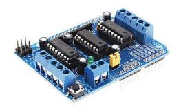
L293D Motor Drive Shield is a monolithic integrated, high voltage, high current, 4-channel driver.
