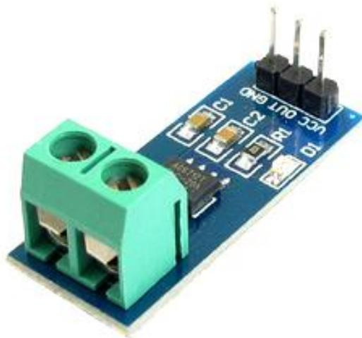
Accurate sensor to measure AC/DC current up to 20A. The sensor can even measure high AC mains current and is still isolated from the measuring part due to integrated hall sensor. The board operates on 5V.
