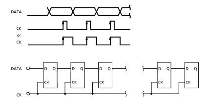
The input data are finally transferred to the latch circuit from the shift register by the ST signal, updating the previous data.
