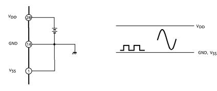
The operating voltage range of a single power supply use is half of a dual power supply use.
