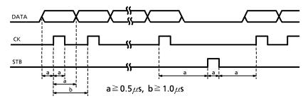
The data to the DATA terminal is input to the internal shift registers sequentially with synchronizing to the rise of the input to the CK terminal.
