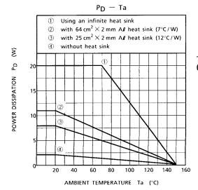
Thermal resistance  $\theta_{ic} = 4^{\circ}C/W$
