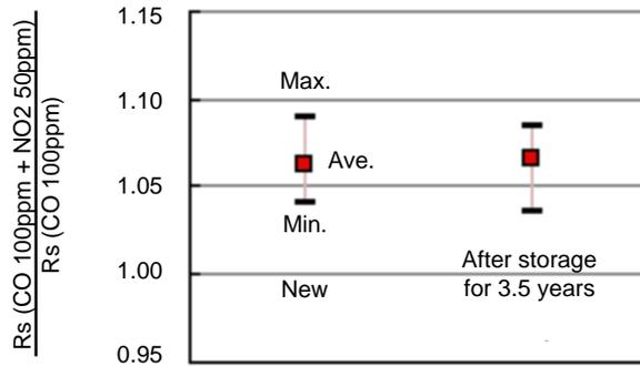
Figure 18 - Effect of being stored in normal air
