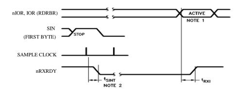
**Note 1:** This is the reading of the last byte in the FIFOs **Note 2:** If FCR0 = 1, then  $t_{SINT} = 3$  RCLKs. For a timeout interrupt,  $t_{SINT} = 8$  RCLKs
