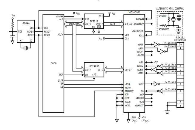
This shows the basic connections of an MC16C550 to an 8088 CPU
