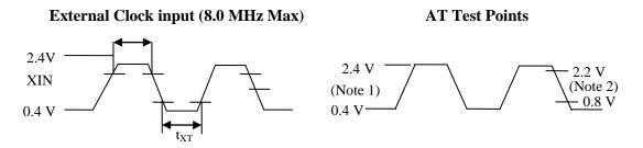
**Note 1:** The 2.4V and 0.4V levels are the voltages that the inputs are driven to during AC testing. **Note 2:** The 2.2V and 0.8V levels are the voltages at which the timing tests are made.
