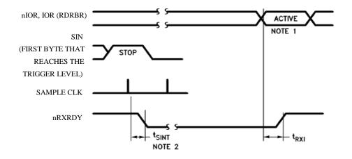
**Note 1:** This is the reading of the last byte in the FIFO. **Note 2:** If FCR0 = 1,  $t_{SINT} = 3$  RCLKs.
