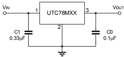
Note 1: To specify an output voltage, substitute voltage value for "MXX".
