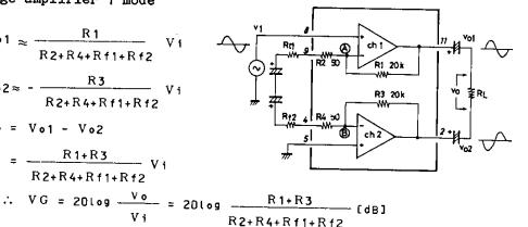
Assuming R2=R4=50ohms, R1=R3=20kohms and Rf1=Rf2, the voltage gain is obtained by:  $VG = 20log \frac{R1}{Rf1+R2} [dB]$
