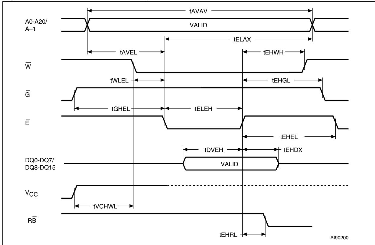
Table 14. Write AC Characteristics, Chip Enable Controlled
