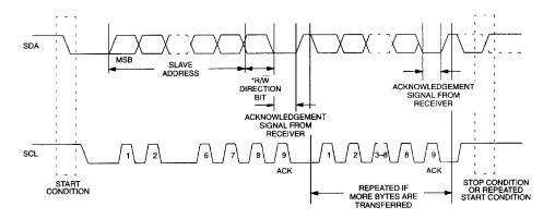
DATA TRANSFER ON 2-WIRE SERIAL BUS Figure 5
