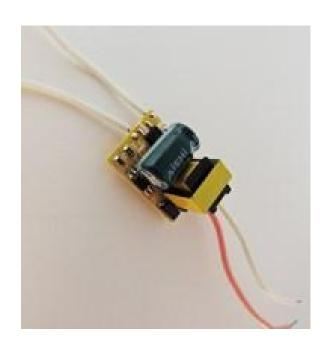
Input Voltage: AC 85-265V Output Current: 300MA<±5%
